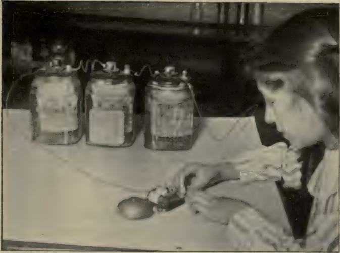
FIG. 111. A wet battery of three cells connected to ring a bell.
